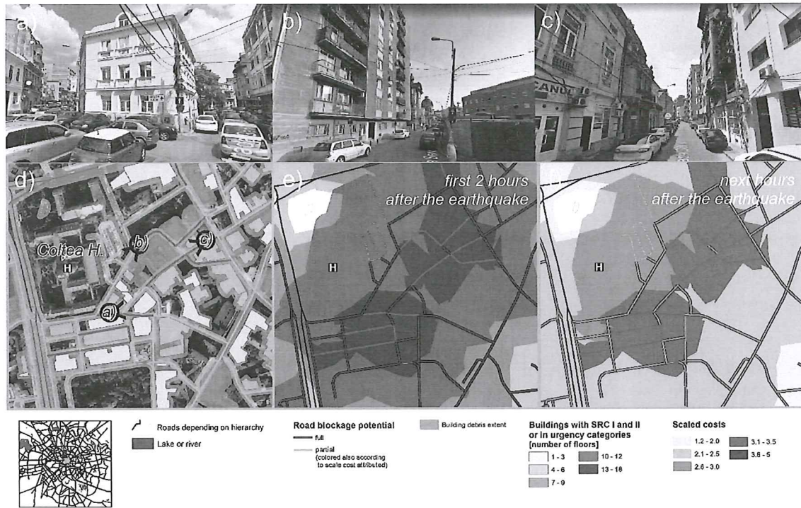
Figure 5 An example of results of the automatic determination of fully or partially blocked road segments due to building debris (d) for a central area near the Coltea Hospital, and exemplification of the real situation (a, b, c – source: Google Street View). Scaled costs calculated using Table 1 are also represented (e and f)
