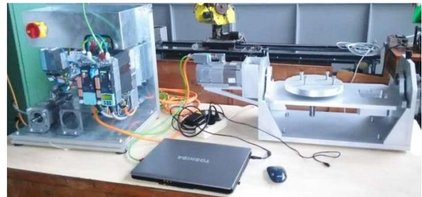
Fig. 1. The experimental system using a rotary table.
