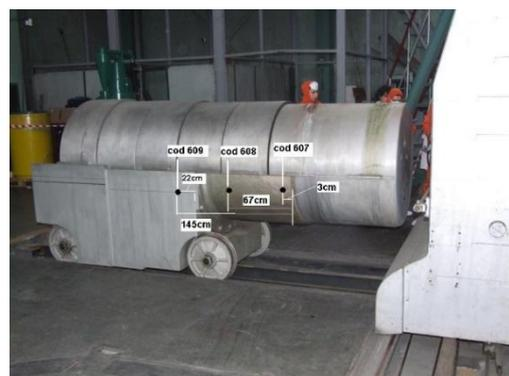
**Fig. 2 - Graphite column made of graphite discs**
