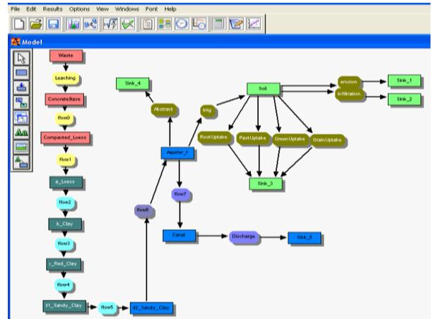
Fig.6 - Repository model used in AMBER 5.5 code.
