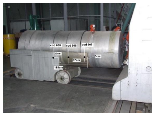
Fig. 2 - Graphite column made of graphite discs
