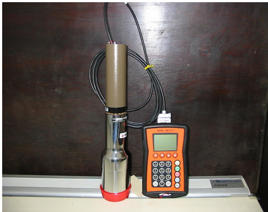
Fig. 12 \gamma Portable Spectrometer - ORTEC, DigiDART
