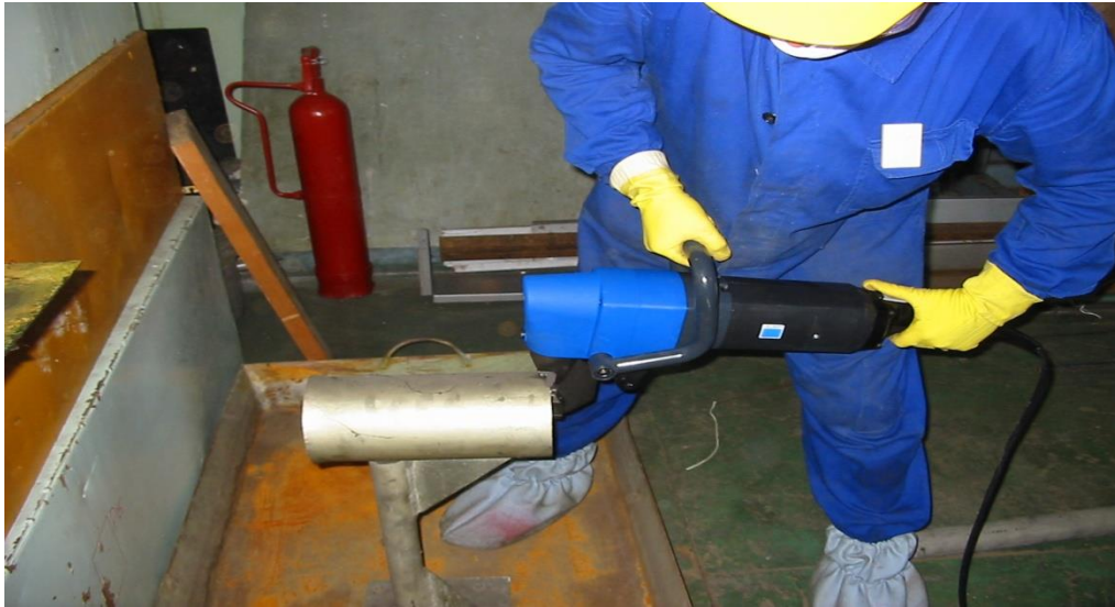
Fig. 6 Device for sampling through stamping, type TRUMPH Nibbler N-1000-0
