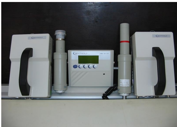
Fig. 9 Universal Monitor, LB 123 “UMo”, type EG&G BERTHOLD
