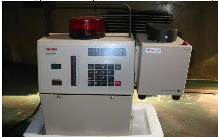
Fig. 11. EBERLINE Monitor for Beta aerosols, type AMS-4
